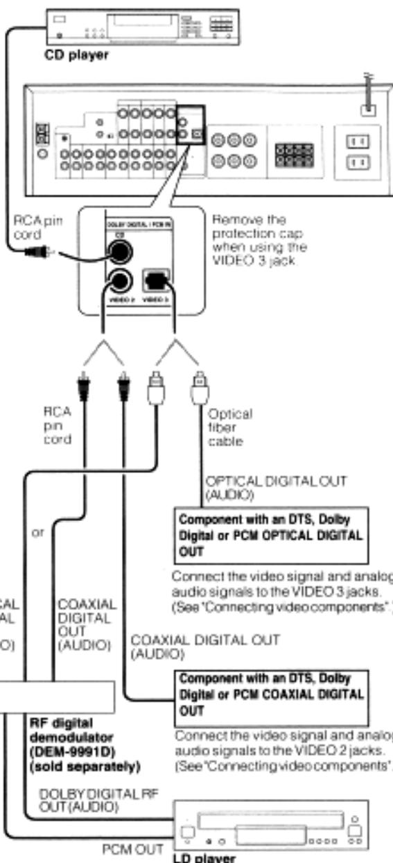
To connect an LD player with a DIGITAL RF OUT, connect the LD player to the KENWOOD RF digital demodulator (DEM-9991D). Next, connect the DIGITAL OUT jacks of the demodulator to the DIGITAL IN jacks of the receiver.
